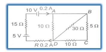
Hints: -equivalent resistance between B and D is 100. It means 0.2 A of
