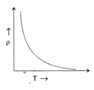
Ans. Resistivity of a semi conductor decreases rapidly with temperature.
